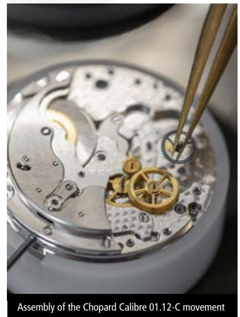
The Chopard Calibre 01.12-C powers the timepiece
